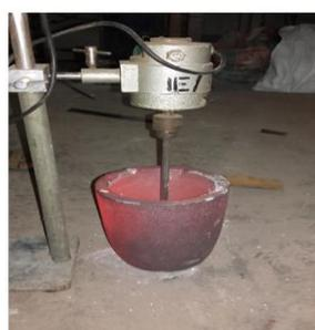
**Fig.2.** Portable electrical motor stirrer
